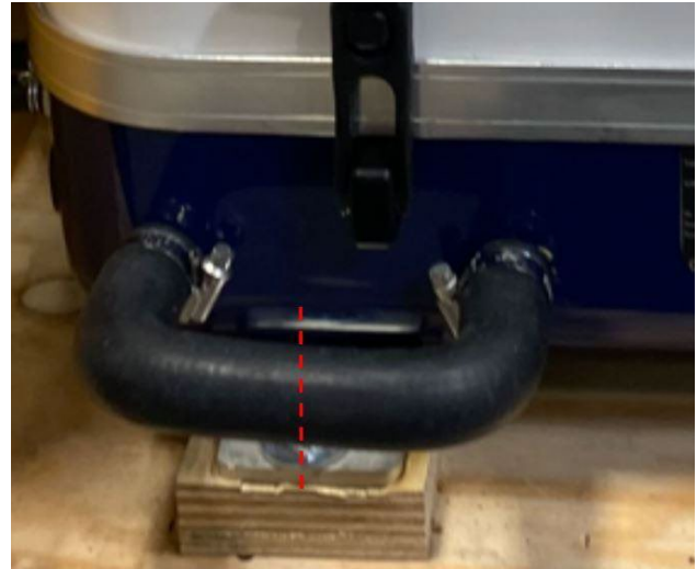
Figure 11: Cutting the Siphon Break Loop
