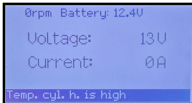
Figure 8: Shutdown Message: Light text with a dark background.
