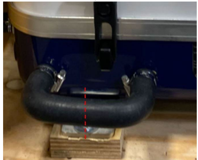
Figure 12: Cutting the Siphon Break Loop
