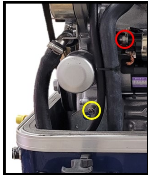
Figure 21: Starter Battery Cable Attachment Points
