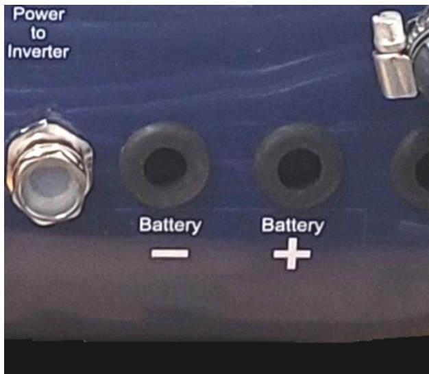
Figure 19: Starter Battery Cable Openings on Capsule
