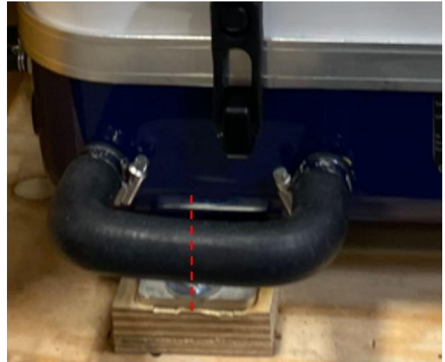
Figure 11: Cutting the Siphon Break Loop
