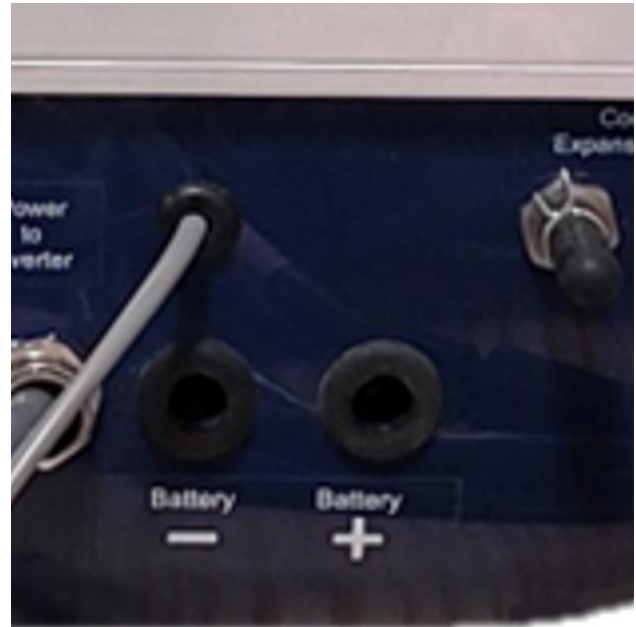
Figure 20: Starter Battery Cable Openings on Capsule
