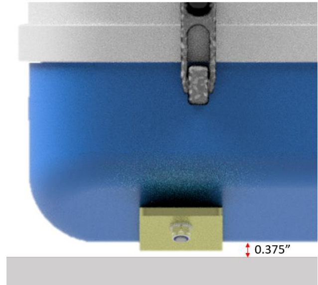
Figure 9: Generator Bottom Clearance
