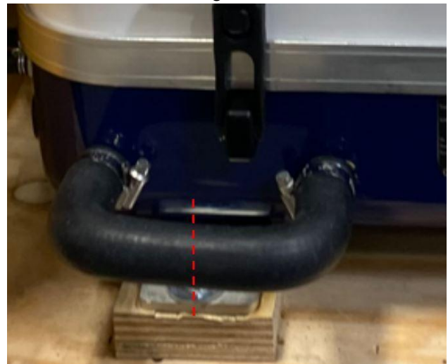
Figure 12: Cutting the Siphon Break Loop
