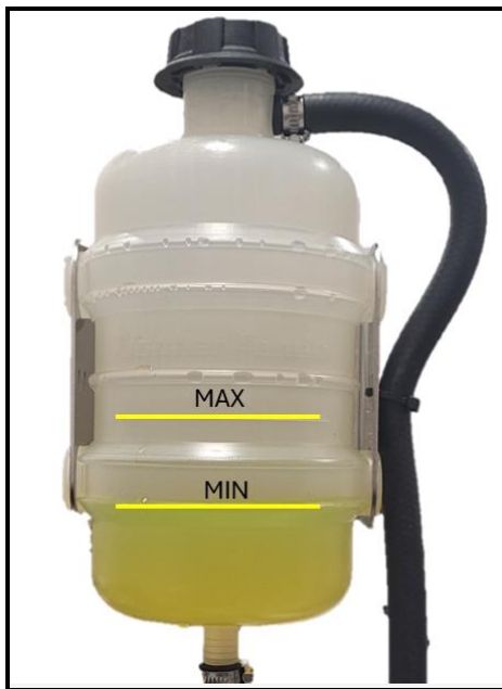
Figure 30: Coolant Expansion Tank
