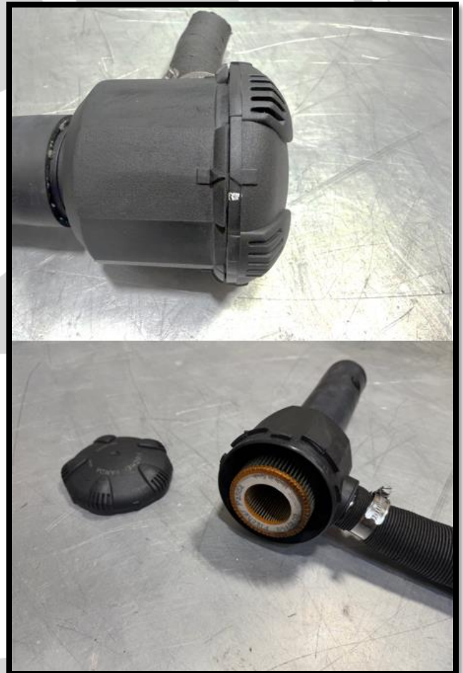
Figure 23: Air Intake Housing and Filter
