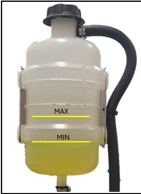
Figure 28: Coolant Expansion Tank
