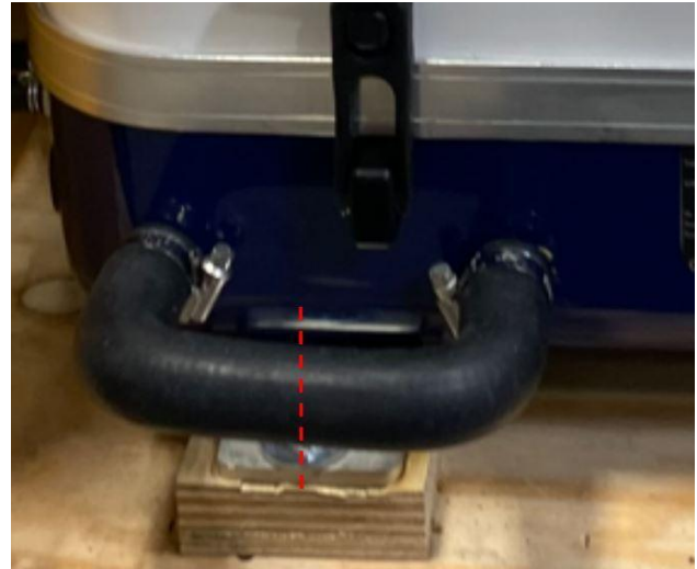
Figure 11: Cutting the Siphon Break Loop
