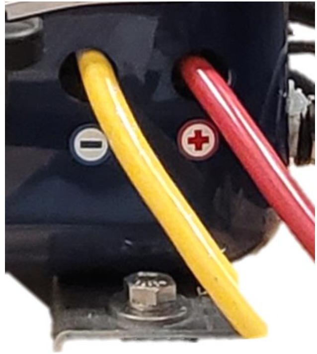
Figure 18: Starter Battery Cable Openings on Capsule
