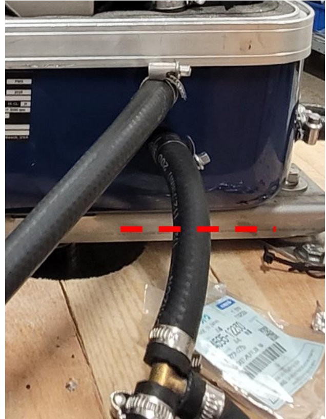
Figure 10: Cutting the Siphon Break Loop
