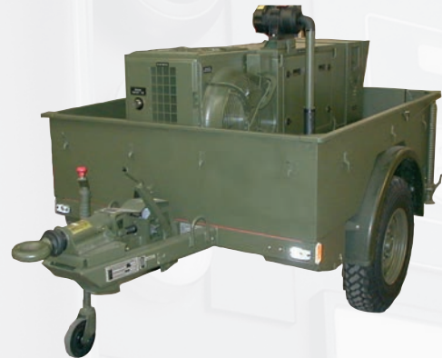
Complete unit, cooling, fuel, generator and electrical systems all mounted on frame. Vertical mounted radiator is rotated 90°, for cooling efficiency in high side trailer.
