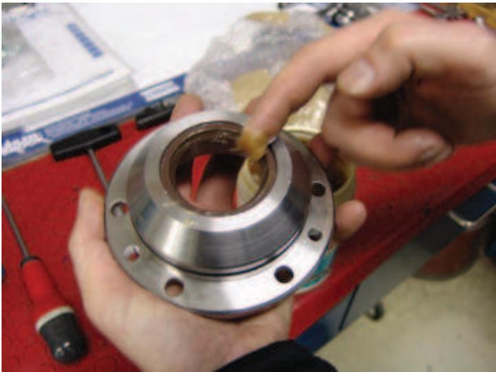
22. When mounting the new bearing housing take care you are not damaging the lipseal while pushing carefully by turning right and left over the rotor. Tighten the bolts
