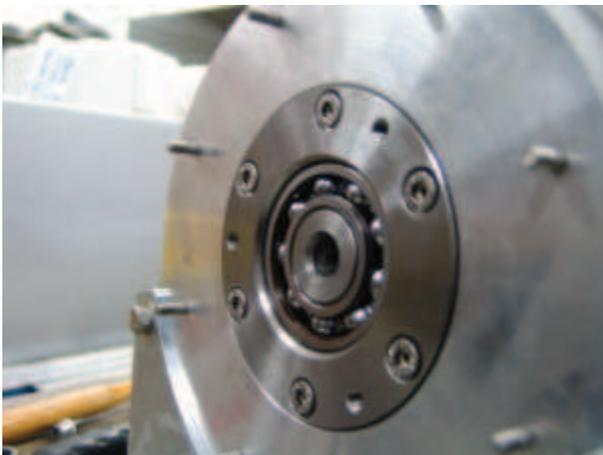
25. Before you mount the lid, grease the o-ring to ensure it will stay in position. Mount the aluminium lid. Take care, that the o-ring is in the right position and tighten the nuts
