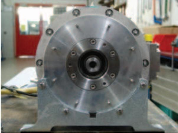
23. Turn a threaded rod into the shaft up to the end
