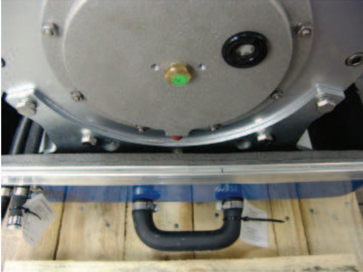
20. Mount the new alternator with winding carefully that way the winding will not be damaged by the rotor and pull it until it fits on the flange position. Insert the bolts at the flange and tighten them.
