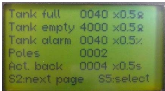
Figure 21: Resistance for tank sensor and alarm level
