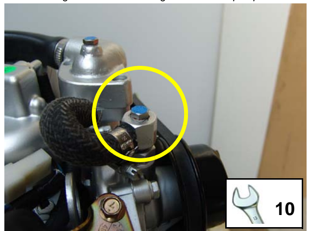
Fig. 4.5.3-3: De-aerating screw - water pump
