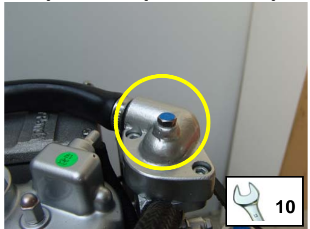
Fig. 4.5.3-3: De-aerating screw - water pump
