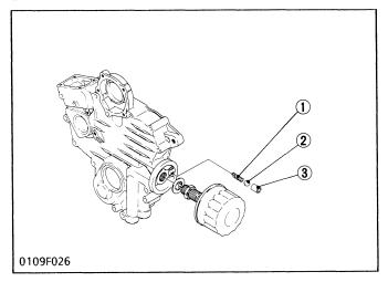
The relief valve prevents the damage to the lubricating system due to the high pressure of the oil.
