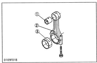
Connecting rod (2) is used to connect the piston with the crankshaft. The big end of the connecting rod has a crank pin bearing (3) (split type) and the small end has a small end bushing (1) (solid type).
