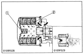
After lubricating, the lubricating oil brings back various particles of grit and dirt to the oil pan. Those particles and the impurities in the lubricating oil can cause wear or seizure of the engine parts. It may also impair the physical and chemical properties of the oil itself
