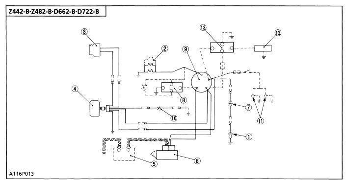
The electrical system of the engine consists of a starting system (including a starter, glow plugs and others), a charging system (including an AC dynamo, a regulator and others), a battery and an oil switch.
