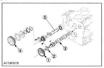
The camshaft (3) is made of special cast iron and the journal and cam sections are chilled to resist wear. The journal sections are force-lubricated. The fuel camshaft (5) controls the reciprocating movement of the injection pump. The fuel camshaft is made of carbon steel and the cam sections are quenched and tempered to provide greater wear resistance.
