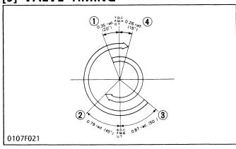
The timing for opening and closing the valve is extremely important to achieve effective air intake and sufficient gas exhaust.
