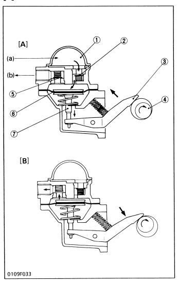
The filtered fuel is fed to the injection pump by the fuel fed pump.
