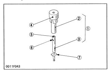
The pump element (1) is consist of the plunger (3) and cylinder (2).
