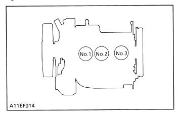
The cylinder numbers of 68 mm STROKE SERIES diesel engine are designated as shown in the figure.
