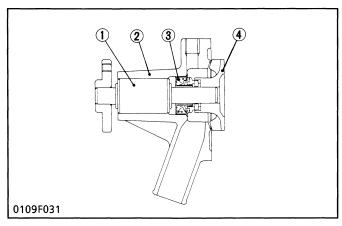
The water pump is driven by the crankshaft via a V-belt. Water cooled in the radiator is sucked into the water pump from its lower portion and is sent from the center of the water pump impeller (4) radially outward into the water jacket in the crankcase.
