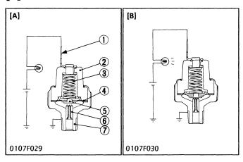
The oil pressure switch is mounted on the cylinder block and is led to the lubricating oil passage.
