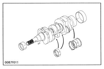
The crankshaft with the connecting rod converts the reciprocating motion of the piston into the rotating motion.
