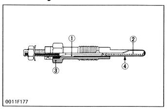
Each sub-combustion chamber has a glow plug for easy starting. The glow plug is of the quick-heating type.
