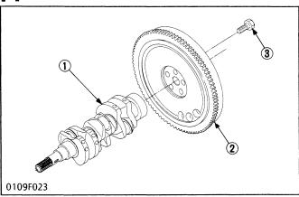
The flywheel stores the rotating force in the combustion stroke as inertial energy, reduces crankshaft rotating speed fluctuation and maintains the smooth rotating conditions.
