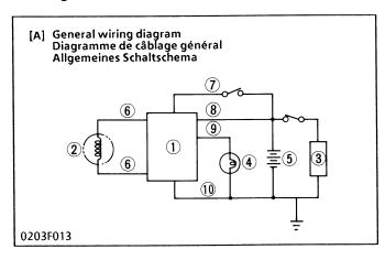
The regulator performs rectification and voltage regulation. The regulator converts AC into DC which flows through the power consuming circuits and the battery, and also charges the battery. If however, the battery voltage exceeds a certain level. The DC current is cut off from the charging circuit to prevent overcharging.
