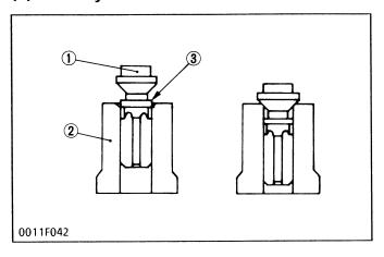
The delivery valve consists of the valve (1) and the Valve seat (2).
