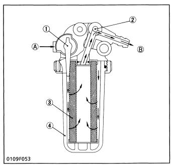
Each moving part of the injection pump and nozzle is extremely precision machined, and clearances of their sliding parts are extremely small. Fuel itself serves as lubricating oil. For this reason, it is extremely important to completely remove water and dirt contained in fuel.
