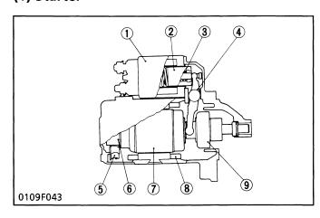
The starter is of the electromagnetic drive type. It is composed of a starting motor and a solenoid switch.
