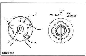
The key switch has 4 positions. The terminal "BAT" is connected to the battery.
