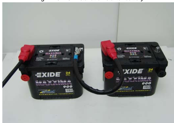
Fig. 7.10.2-3: Installation starter battery
