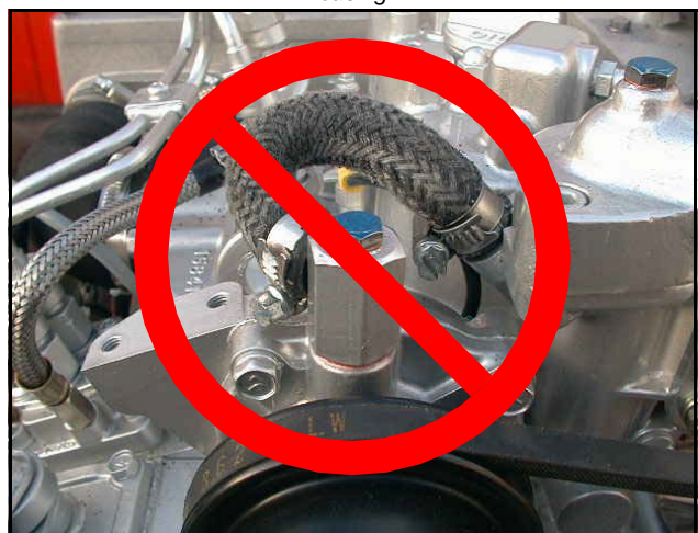
Fig. 8.10-5: Ventilation screw above the cooling water pump casing
