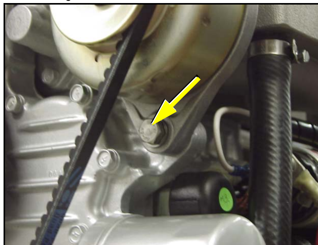
Fig. 8.10-2: Screw underneath the alternator
