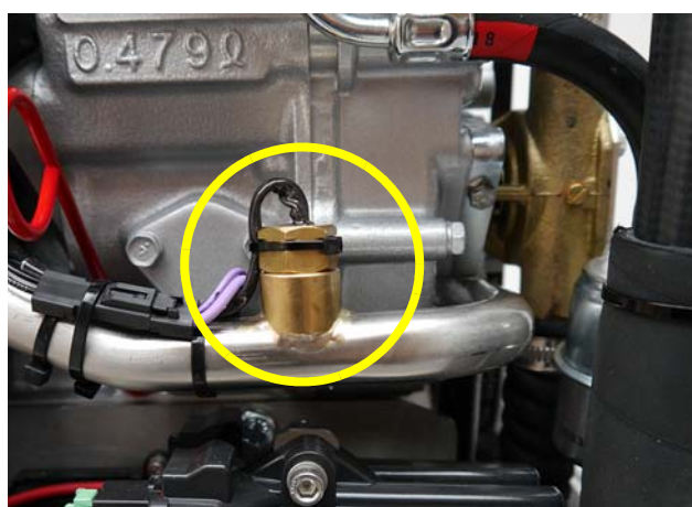
Fig. 5.2.4-3: Thermo-sensor raw water in
