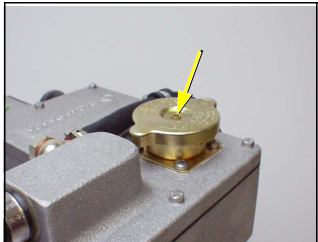
Fig. 8.10-4: Cooling water filler cap
