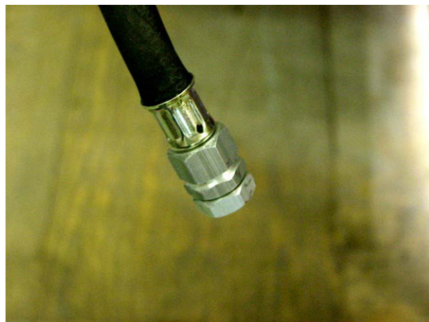
Fig. 8.8-2: Oil drain hose
