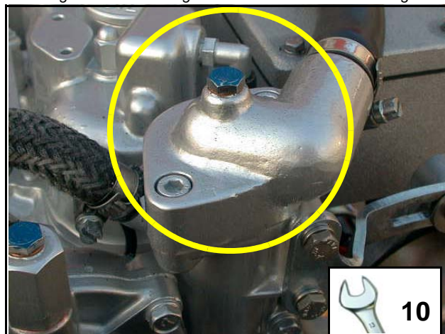
Fig. 5.15.1-3: Venting screw at the thermostat housing
