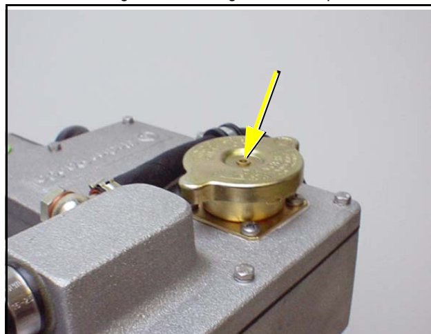
Fig. 6.10-4: Cooling water filler cap
