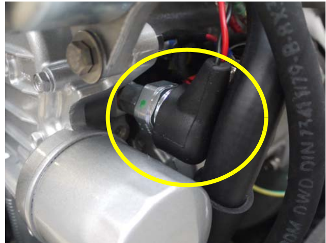
Fig. 3.3.4-4: Oil pressure switch
