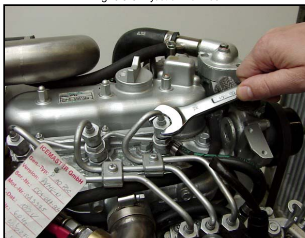
Fig. 6.9-3: Injection nozzles
