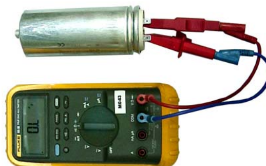
Fig. 6.13.2-3: Capacitor checking
