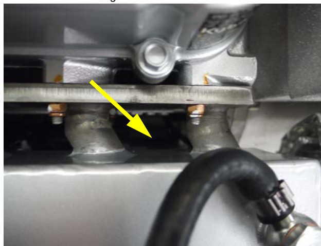
Fig. 6.14-7: Electric starter
