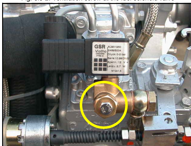
Fig. 6.9-2: Ventilation screw at the fuel solenoid valve
