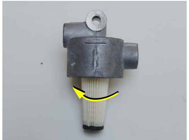
Fig. 6.9.1.1-3: Fuel filter
