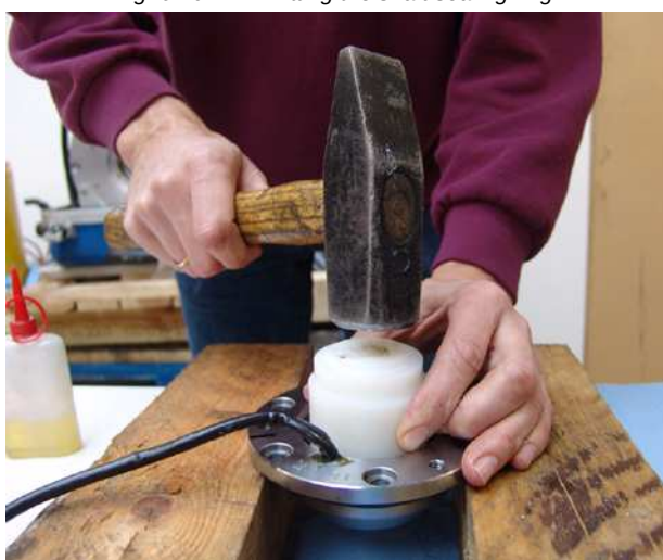
Fig. 6.10.2-17: Fitting the shaft sealing ring
