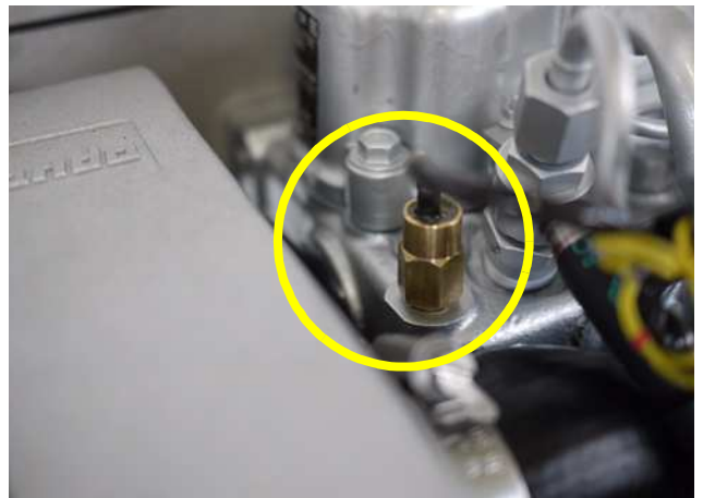
Fig. 4.3.7-1: Thermo-switch at cylinder head
