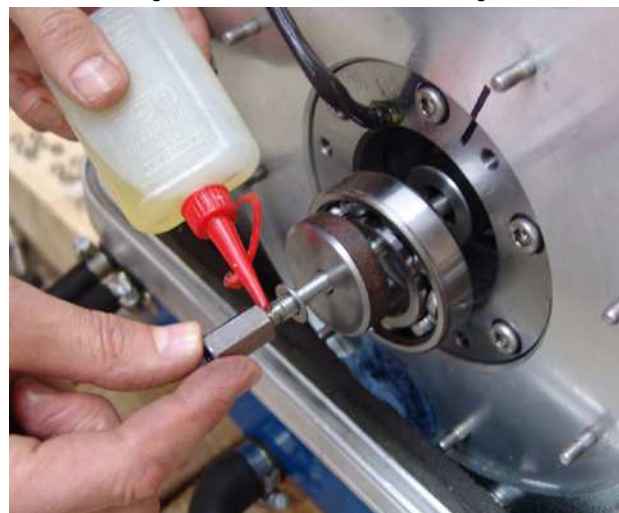
Fig. 6.10.2-26: Mount the ball bearing
